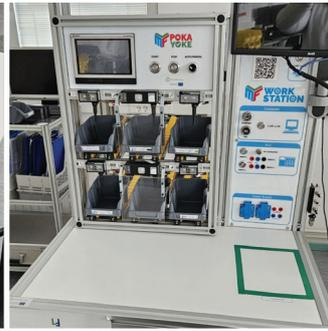
Figure 3. Poka Yoke Assembly Station
